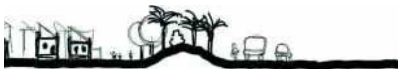
Topography can also be effectively used to buffer or shield the community from unwanted features
